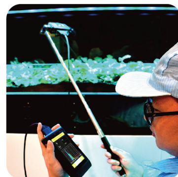
Sensor head can be used with a selfie stick and camera tripod. Users can easily measure far reaching ranges and adjust the measurement point horizontally.
